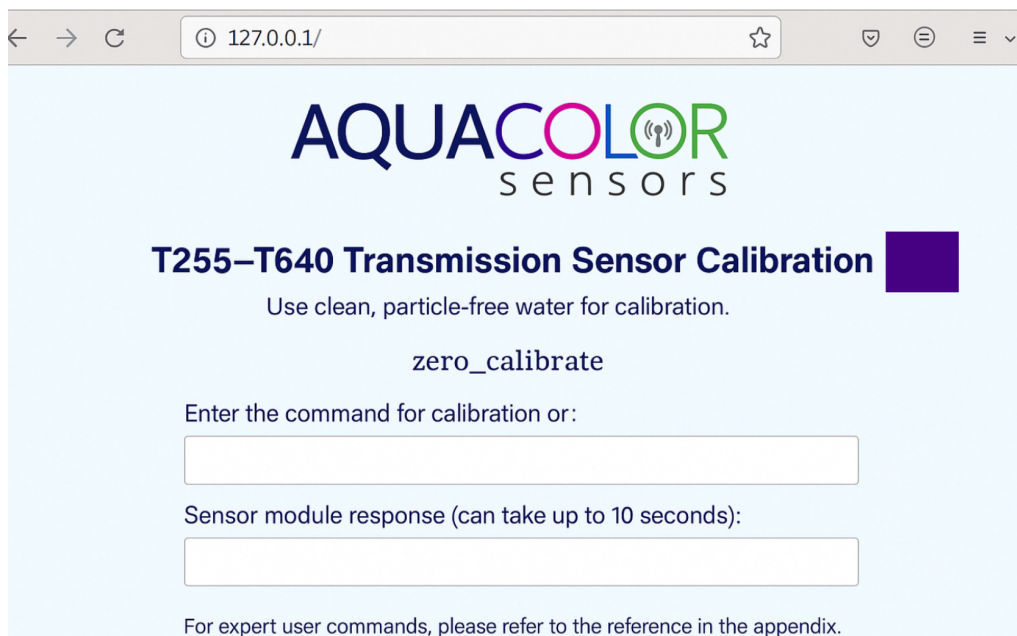
Figure 11: Calibration interface for the T255–T640 transmission sensor.
