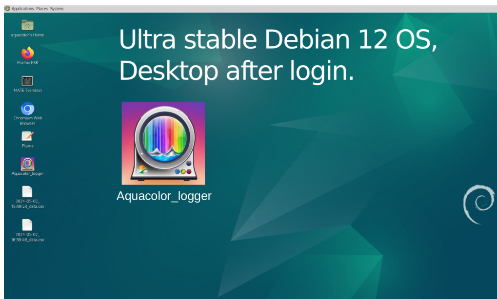
Figure 3: Login screen showing the Debian 12 desktop with the Aquacolor.logger application icon magnified. Clicking the icon will start the aqua.logger's GUI.
